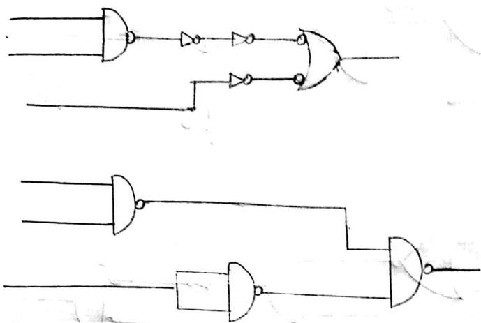
$$f = \overline{(A+B) \cdot C \cdot D} \quad f = \overline{(A+B) \cdot C} \cdot D \quad \text{using only NOR gates}$$
